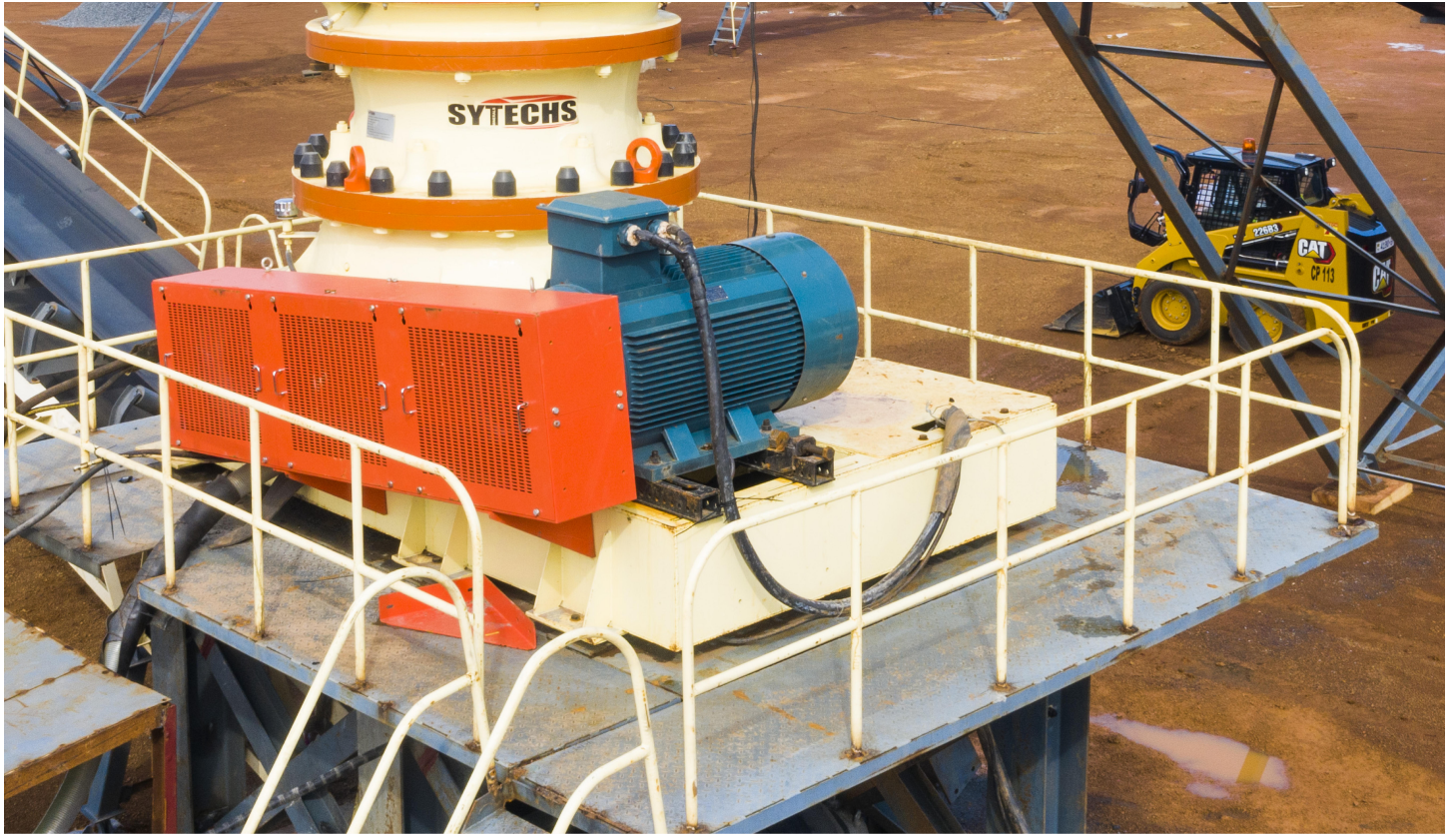
Skid mounted Unit. The cone crusher along with the driving electric motor are both mounted on a skid structure to reduce vibration and belt hammering. This results in better driving performance and longer motor bearing/counter shaft bushing life.
